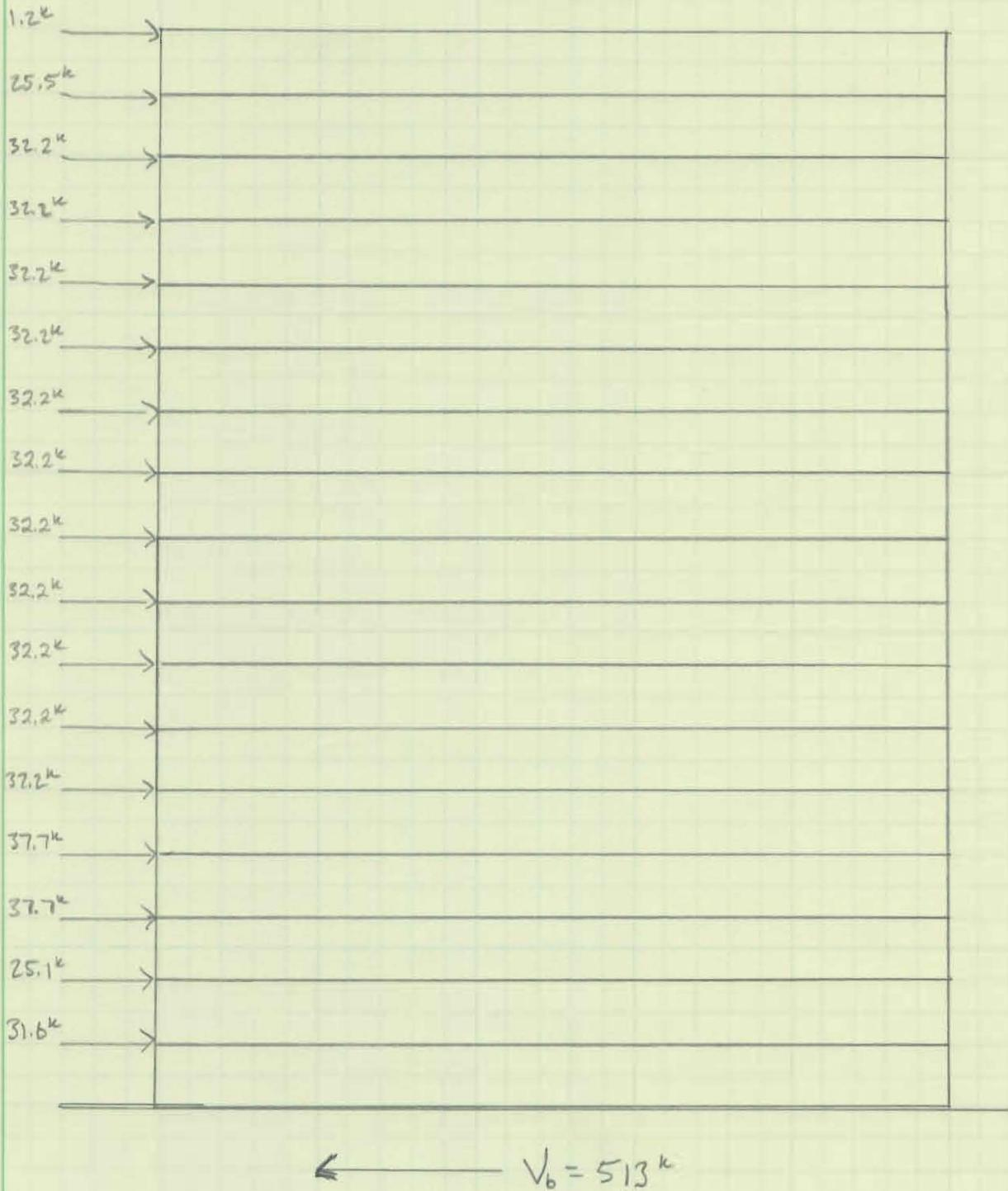
Seismic Story Forces - E/W, in kips
