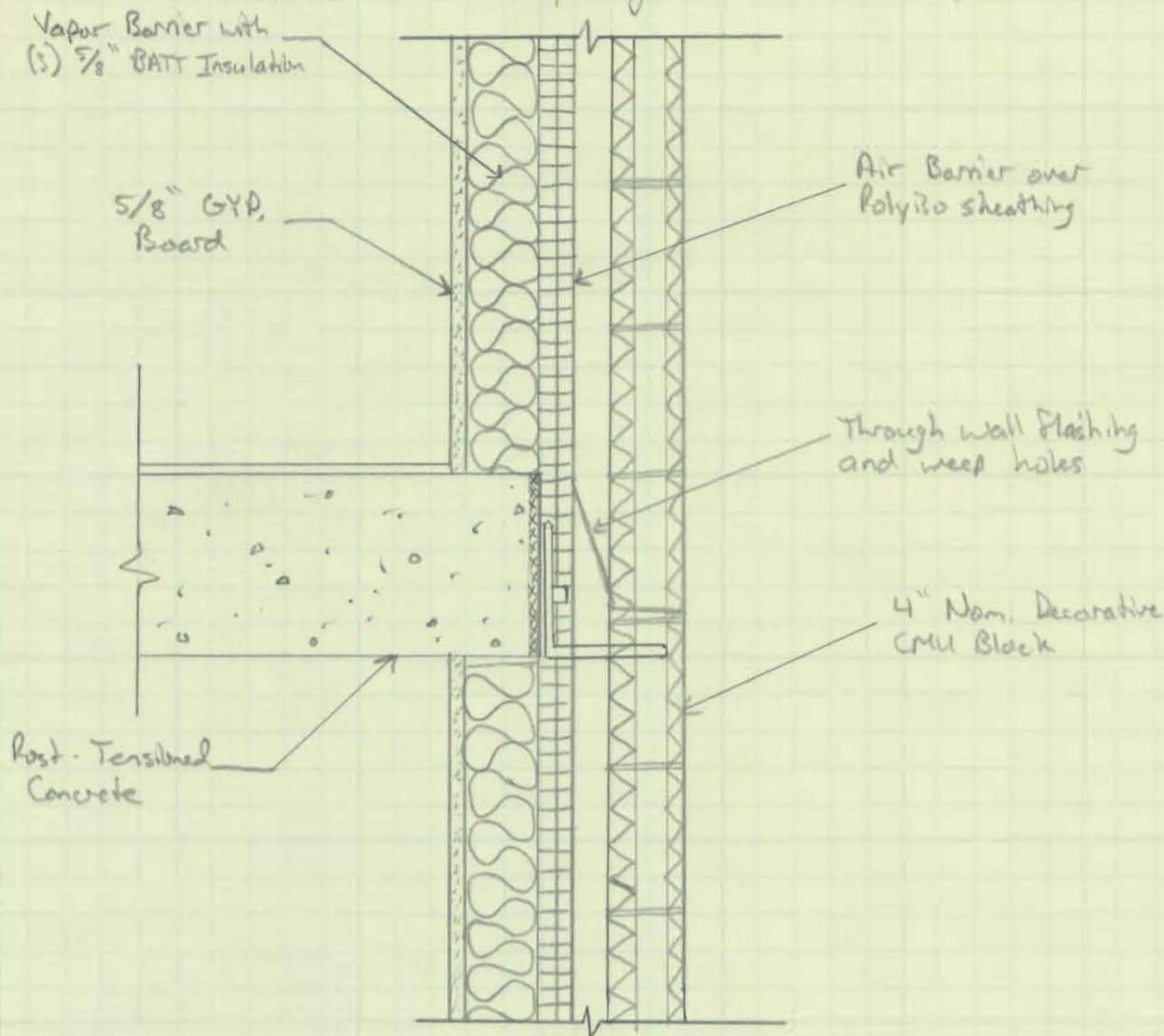
Gypsum Board -  $\frac{5}{8}'' \times 4 \frac{\text{psf}}{\text{in}} \times 10' = 25 \text{ pif}$
